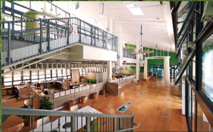
Cross ventilated open plan layout
